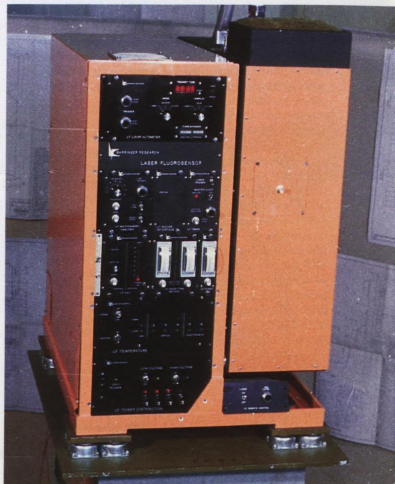
Mark III airborne laser fluorosensor system.
