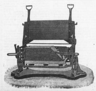
This Machine makes all blocks face down-"the only practical way '-allowing of a richer and finer facing, producing blocks that are perfect in appearance and impervious to moisture.
