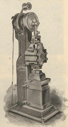
allowing the operator to lengthen or shorten the stroke at will. Motion is applied to the head or ram, by means of a circulating rod in a sleeve or collar supplied with a large set-screw, or, as in the large sizes, a clamp to hold the rod in position, and to this sleeve are hinged two side arms, these in turn being connected to the ram by metal links. By the use of a steel spiral spring, carefully adjusted between these arms, the force and weight of the blow are many times
