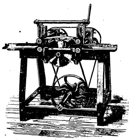
This machine carries four 12 inch saws, and is fitted throughout for continuous, fast work. The frame is a solid iron casting with long bearings for saw arbor cast in place. So it is impossible for the arbor ever to get out of line. The drive pulley on arbor is 8 inch dia., 9 in. face, turned inside and out and firmly balanced.
