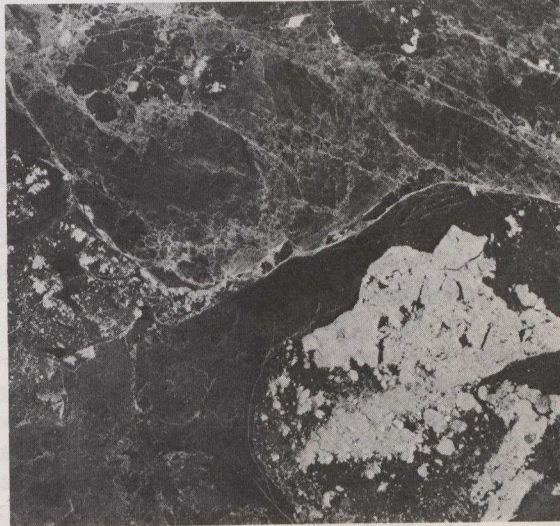
Star-1 synthetic aperture radar image of ice fields in the Beaufort Sea made from more than 9 000 metres above and transmitted to a ground station by digital data downlink shows ice types, small multi-year ice hazards, pressure ridges, ice breaker tracks and drilling vessels.
