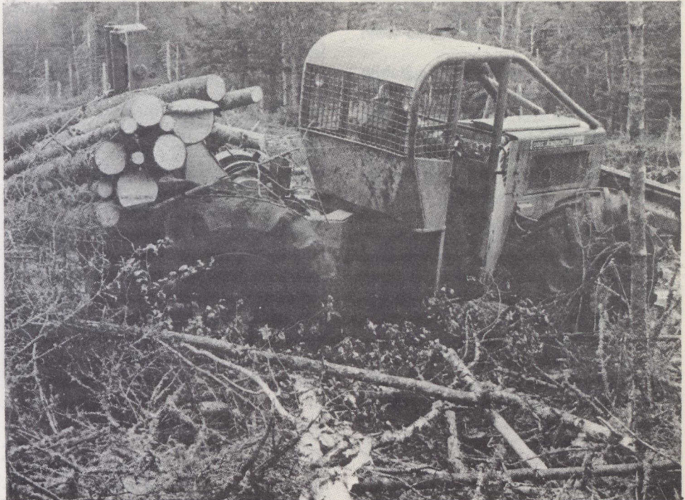
A "skidder" plows through heavy underbrush with a pile of eight-foot logs.
