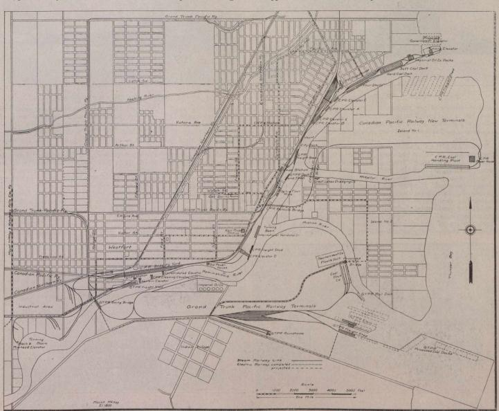
Fig. r.-Plan Showing Railway Connections Around Fort William.
