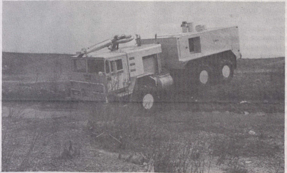
Although the fire truck weighs 22 tons, its soft tires exert one-quarter the pressure a square inch of regular truck tires. (Above) the truck rambles over soggy terrain.
