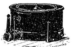
Direct Steam Driven. No Shafts or Belting required. Suspended on Links and requiring no Foundation.
