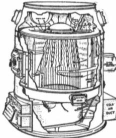
The peculiar construction of the zig zag heat tubes enables The Kelsey to generate an enormous quantity of air at a moderate temperature rather than a small amount of air intensely hot and really poisonous.
