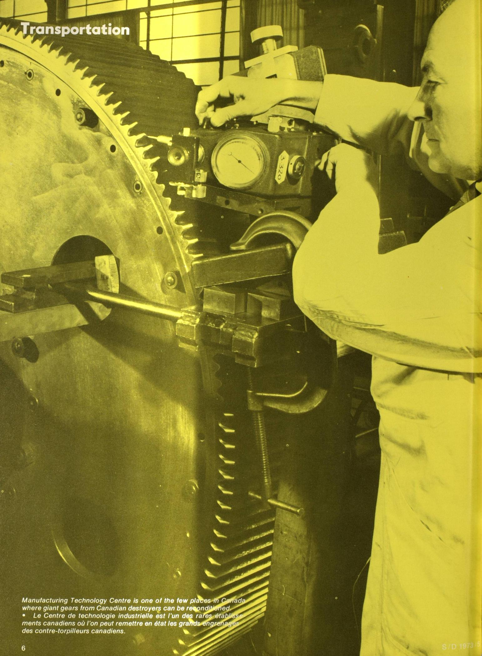
Manufacturing Technology Centre is one of the few places in Canada where giant gears from Canadian destroyers can be reconditioned.
