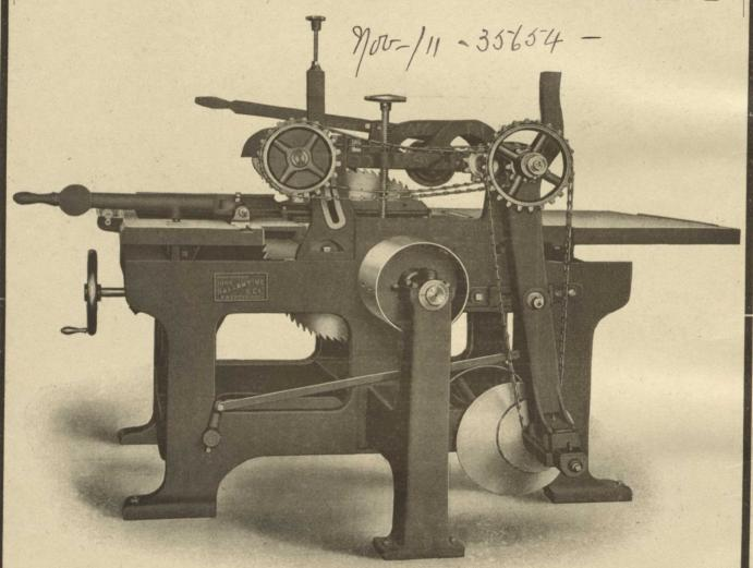
Our No. 2 Variable Self-Feeding Rip Saw. Feed varies from 0 to 200 feet per minute. Weight about 3,000 lbs.
