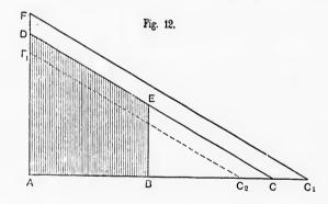
and BE represent the spring force corresponding to positions A and B of weight-arm. Assuming perfect isochronism between weight and spring, then AD and BE also represent the balanced centrifugal force, and this force for any intermediate position of weight-arm is the corresponding height from the line AB to the line DE. Up to this time we have neglected the effect of valve-gear friction.
