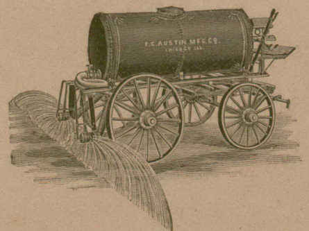
AUSTIN STEEL STREET SPRINKLER
