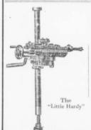
This machine shears or undercuts with equal facility.
