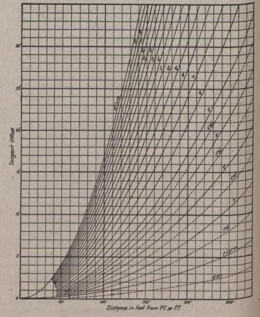
If used in connection with a well-arranged set of tables of the one degree curve, such as Table. 30 in "Harger and Bonney's" handbook, it will practically eliminate figuring in the field and speed up the survey considerably.
