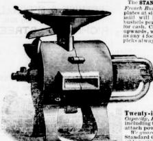
The STANDARD 12 inch CHOPPER uses besi French Burr Mill Stones. No removing of iron plates at six dollars per pair. Stones in this mill will last a lifetime. Capacity, 5to 15 bushels per hour. Price \$85.00, less 10 per cent for cash. Can be driven by 2 horse power and upwards, will grind any kind of grain as fine as any 4 foot run of stones. 2 English steep picks always with each mill. Easily kept order
