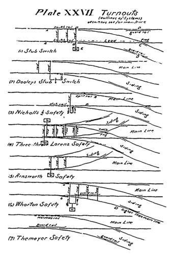
throat of the frog. The stub switch works for a threethrow as easily as for a two-throw turnout, and can be made into a safety switch (see Cook Switch, Plate XXVII., and Dunn Switch, Engineering News, Vol. II., 1890, page 174), and is considered to be more durable and easily kept in working order with snow and ice than are the many forms of split rail switches.
