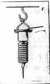
SPRING GIVES NEEDED TENSION. vishes to tie up a bundle he uses the wine just as if he was unrolling it rom a ball, but the spring provides ust the tension necessary to facilitate the work. If you will stop to think you will recall that it is much easier to tie a package when the cord is fed out from its source of supply
