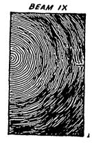
to date would seem to indicate that the best classification defining the strength of the timber would be found by dividing the section of a log into three parts by means of two circles, with the heart as the centre, and by designating the central portion as 3rd quality, the portion between the two circles as 2nd quality, and the outermost portion as 1st quality.
