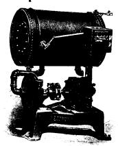
Increases rapidity of circulation by grawing condensation through the system, venting the air and returning water to boiler at high temperature. Eliminates snapping, pounding and cracking in radiators and pipes. Comprised of an expansion tank, automatic switch and centrifugal pump automatically operated by electric motor. Easily installed and increases the efficiency of either high or low pressure system 50 per cent.
