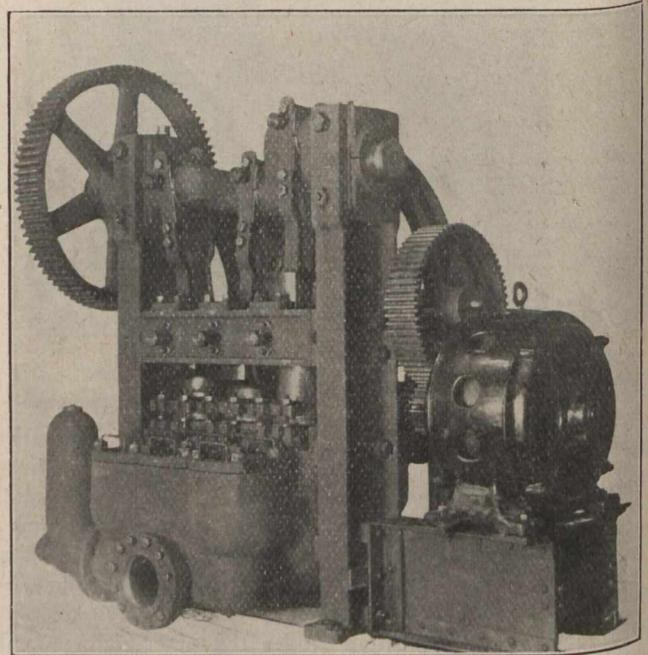
built so that the speed of the water, as it passes through the pump, is about three feet per second. It is maintained that there is approximately 13 per cent. variation in volume of water passing through a pump; consequently, the suction and discharge pipes of these pumps are fitted with chambers which equalize the flow to a uniform speed.
