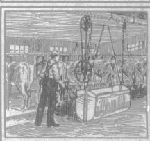
It is a very different matter with a BT Manure Carrier. There is no heavy pushing, no planks to lay, no snow to shovel. The work is done in half the time. If the yard is muddy or filled with snow, it doesn't matter because the overhead track is independent of conditions on the ground.
