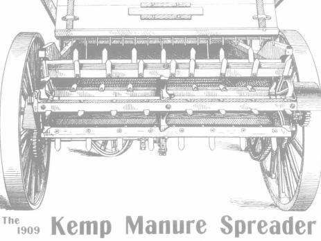
Equipped with the Reversible, Self-sharpening, Graded Flat-tooth Cylinder. The latest improvements of J. S. Kemp, the inventor of the first Manure Spreader. The result of 34 years in the use and manufacturing of Manure Spreaders. Send for our catalogues, fully describing this machine, and also our Imperial Horse-lift Drill. The only drill equipped with a horse-lift.
