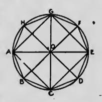
square in the circle. Through the centre, using parallel rulers, draw diameters parallel to the sides of the square. The quadrants are thus bisected, and we get eight equal angles at the centre. Joining ends of the successive radii which bound these angles, we have an octagon inscribed in the circle. The accuracy
