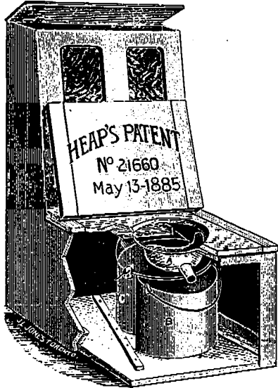
INODOROUS PORTABLE BEDROOM COMMODO A—Urine Separator. B—Urine Receptacle. C—Excrement Tank.
