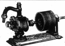
ROTARY FEED PUMP, MOUNTED ON IRON FRAME.
