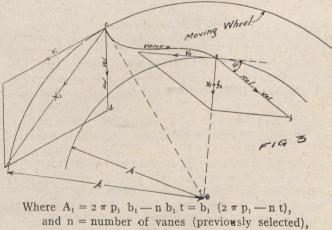
t = thickness of vanes: ¼-in. to ¾-in. for steel and ½-in. when cast.
