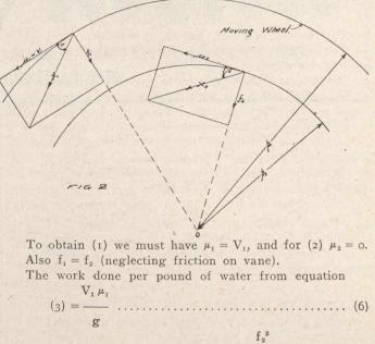
20  $V_1 \mu_1$ Then H = g And since  $\mu_1 = V_1$ , V1  $f_{2}^{2}$ Therefore, H =+ g 2g Since  $\Omega$  = augmented velocity of wheel, V<sub>1</sub> V<sub>2</sub> therefore,  $\Omega = - - =$ p1 p2.  $\mathbf{p}_2$ Therefore,  $V_2 = -$ .  $V_1 - 0.6 V_1$  say.
