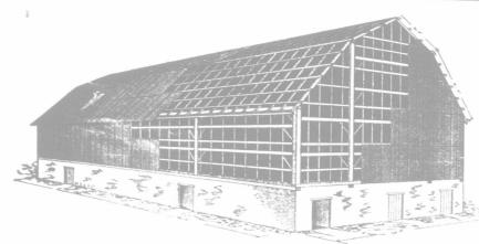
This cut shows an up-to-date Barn Construction, 40 feet x 70 feet, and the method of covering with Corrugated Sheets. The framework is light, as the corrugated sheets, when nailed in place, make the building very rigid. This drawing is made from actual plans and the barn has been built many times with splendid results.
