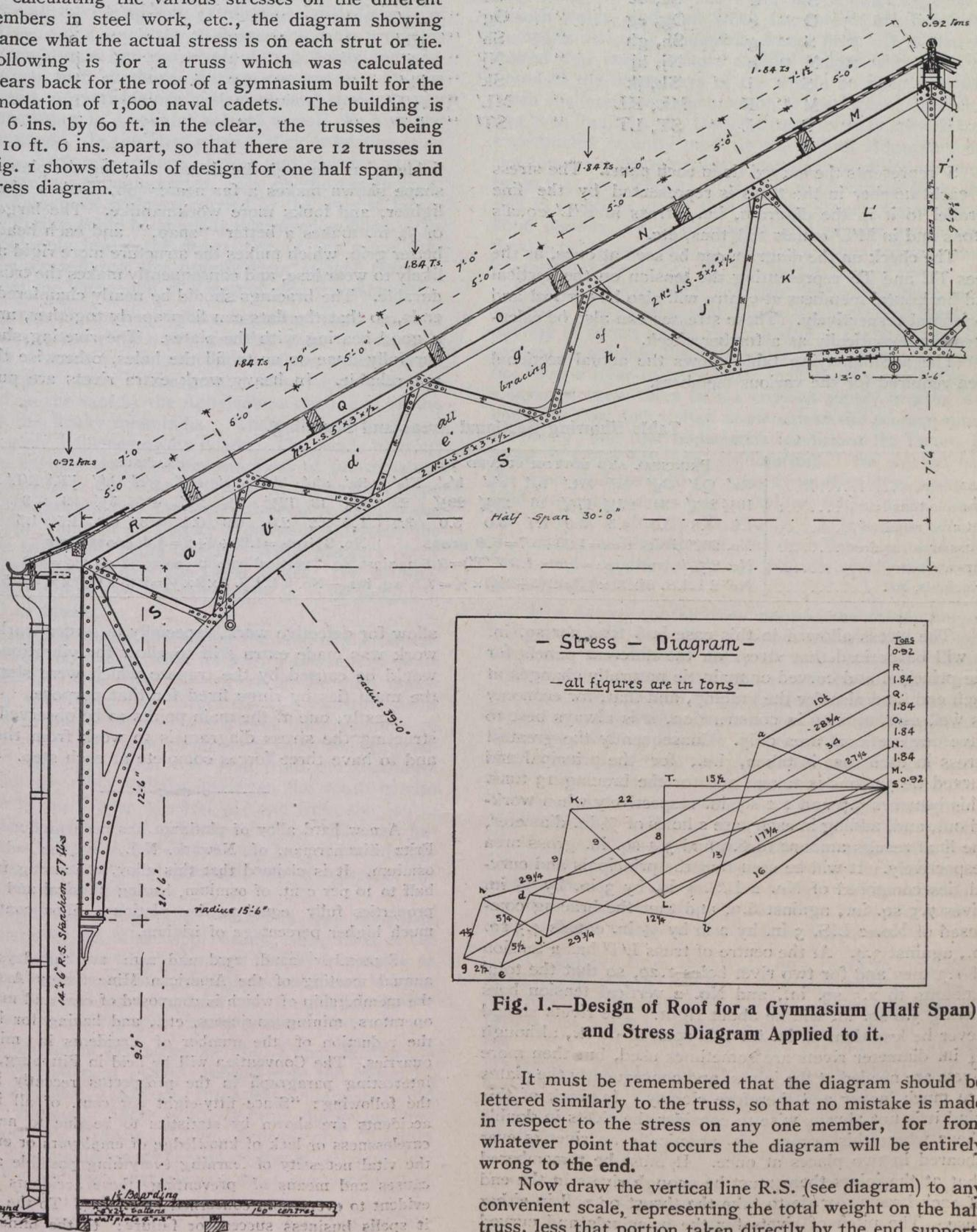
**Fig. 1.—Design of Roof for a Gymnasium (Half Span) and Stress Diagram Applied to it.**
