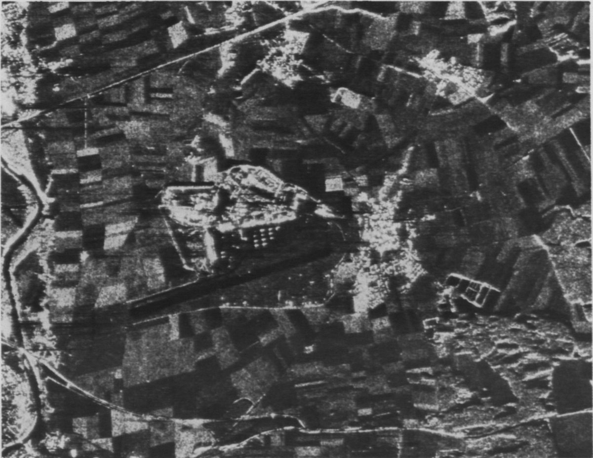
Figure 3. This synthetic aperture radar image was acquired from an altitude of 11,000 metres. Note the broad area coverage provided by SAR and the reflective characteristics of the vehicles, perimeter fence and buildings. The spatial resolution of this image is approximately six metres.
