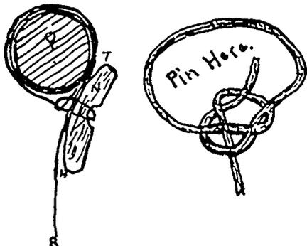
Much difficulty is usually found to hold ropes by means of knots when great stress is applied. By means of the "bowline" knot, a sketch of which is given, we overcame this trouble.
