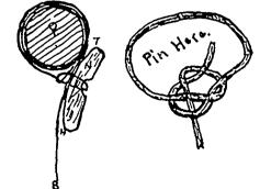
Much difficulty is usually found to hold ropes by means of knots when great stress is applied. By means of the "bowline" knot, a sketch of which is given, we overcame this trouble.
