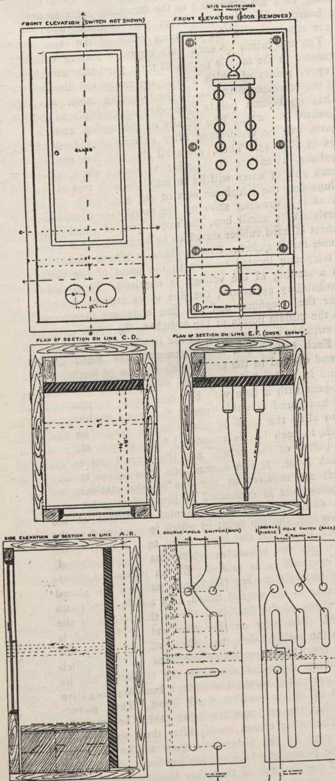
Fig. 16.—Station Switch and Fuse Boxes, Testing System.
