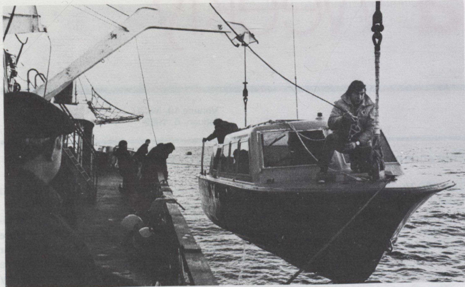
A hydrographic survey launch is hoisted aboard the CSS Hudson in the western Arctic's Beaufort Sea. It is one of five used to survey a safe navigational corridor in the Beaufort.
