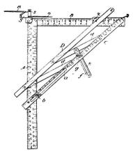
A device for indicating the side cut of rafters comprising a rule or bar adapted to have its edge placed on the plumb cut of the rafter, as indicator plate pivoted to the said bar, to swing at right angles to its length, the said plate having indicating lines marked from a common centre thereof, and fingers pivotally connected with the said plate at opposite sides of the pivotal point and adapted to swing in a plane at right angles to the said plate.
