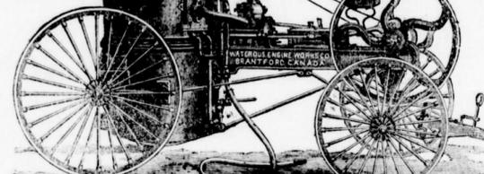
The sectional safety boiler is manufactured expressly for the "North West" trade. This boiler is so arranged that it is readily taken apart in sections enabling purchasers to clean thoroughly every part of it and prevent burning out. We have found that this is absolutely necessary with the alkaline waters of the great Western provinces. Largely used by the Pacific Railway Company and all the large Colonization and Ranching Companies.
