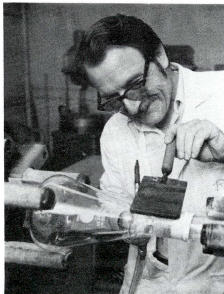
Robert Ducourneau, Agriculture Canada's only scientific glassblower, fuses the neck on a flask. Mr. Ducourneau makes glass apparatus for Research Branch laboratories across Canada.
