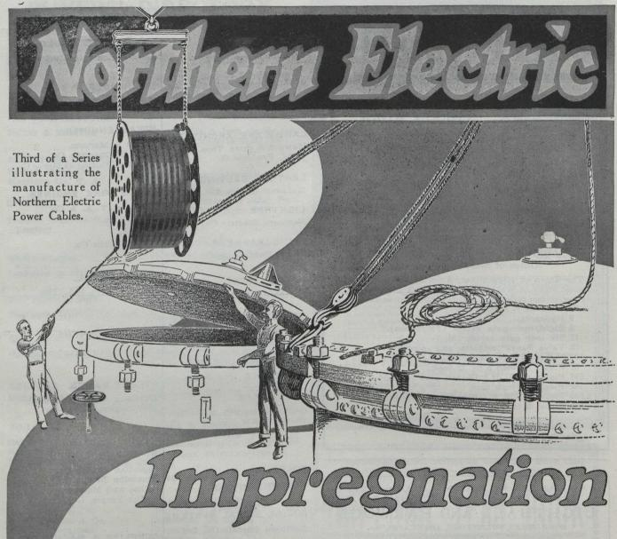
HE Paper Covered Cable is retained at a high temperature in a drying oven until all moisture is eliminated. It is then placed in a steam heated air-tight impregnating tank in which a vacuum is produced to remove all traces of air and moisture. The cable is flooded with hot compound and great pressure applied until the paper covering is thoroughly saturated.
