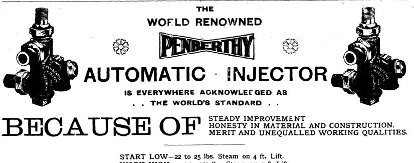
START LOW = 22 to 25 lbs. Steam on 4 ft. Lift. WORK HIGH = 145 to 150 lbs. Steam on 4 ft. Lift. LIFT WATER = 20 ft. on 60 to 80 lbs. Steam. HANDLE HOT WATER = 120° to 125° at 80 lbs. Steam. " " " - 112° to 115° at 100 lbs. Steam. " " 95° to 100° at 125 lbs. Steam.
