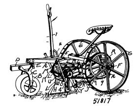
and the frame I, upon which the front end of the grate is supported, combined with the endless carrier L, M, having its rear end journalled in the slotted portion T, so as to be automatically adjustable at this point and mechanisms for operating the carrier and the grate substantially as shown.
