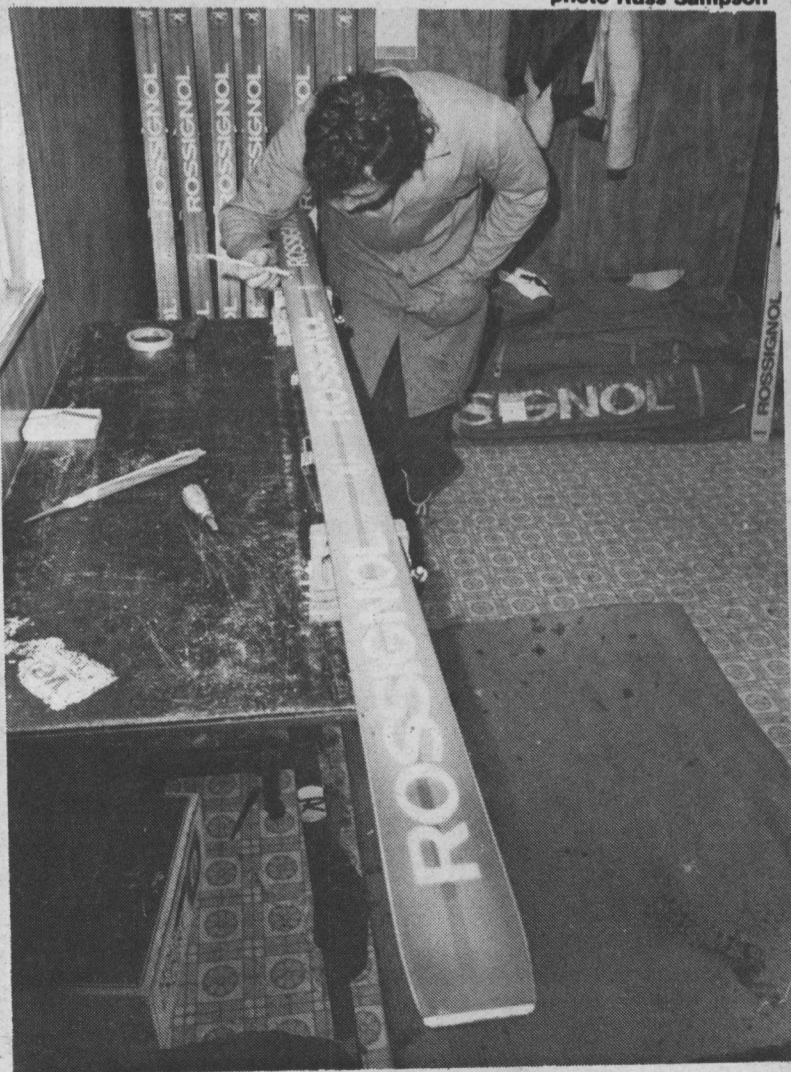
Martin Geofory repairs damaged ski bases on one of racers' many pairs.
