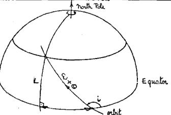
$\sin (\omega + \Theta) = \frac{\sin L}{\sin (180 - b)}$   $\sin (\omega_f + \Theta_f) = \frac{\sin 5 - 205}{\sin 80 - 48}$  = 5.28Since  $\omega_f = 0$ ,  $\Theta_f = 5.28$
