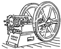
A handy, inexpensive, easily operated motor specially adapted for electric light or pumping service. Special features are. Gets up speed in less than a minute, anyone can manage it and it operates for hours without attention, using fuel in proportion to work done Uses either Illuminating or Natural Gas or Gasoline for fuel.
