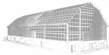
This cut shows an up-to-date Barn Construction, 40 feet x 70 feet, and the method of covering with Corregated Sheets. The framework is light, as the corrugated sheets, when nailed in place, make the building very rigid. This drawing is made from actual plans and the barn has been built many trues with splendid results.
