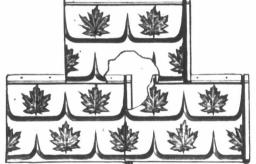
We are manufacturing new Patent Metal Shingles, so constructed that they interlock each other on all four sides, making it impossible for snow or rain to get up under the shingles.
