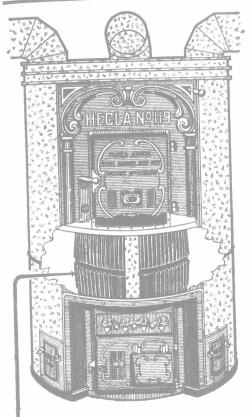
THE HECLA will do this: It is built to save coal at every point, but the big coalsaving feature is the Steel Ribbed Fire Pot. By adding Steel Ribs to the Fire Pot the surface which radiates heat is increased three
