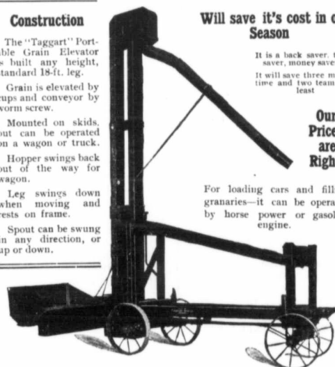
This cut shows Elevator mounted on truck, with leg up and hopper ready to receive grain. Write for prices and terms. Agents wanted.
