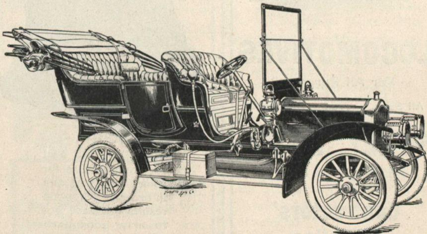
**THE RUSSELL** Built for Canadian roads on Canadian honor. Embodies the latest features of automobile excellence—metal-to-metal disc clutch—shaft drive—selective sliding gear transmission—engine under bonnet—powerful double set of brakes on rear wheels—nickel steel in all gears and shafts.
