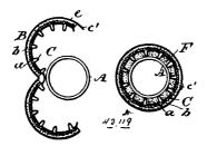
jacket and the pipe upon which it is mounted, of the end collars M, formed by bending fluted sheets of metal into circles, the said collars having the struck up wings E, adapted to engage the ends of the jacket, and the non-conducting fillings interposed between the end collars and the pipe on which the covering is mounted adapted to create a dead air space within the jacket between the end collars, substantially as and for the purpose set forth.
